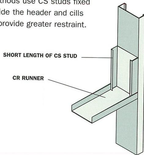
Header and Cill member attached by cutting flanges at 45 degrees and screw-attaching to full height stud.
