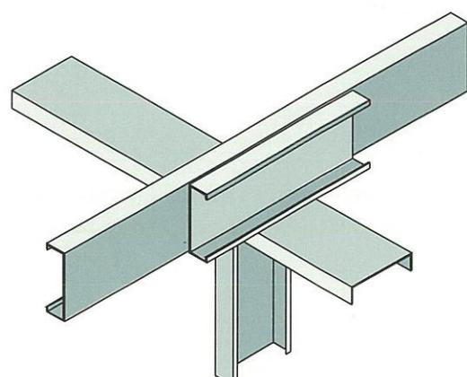
**Joist reinforcement over load bearing wall**
