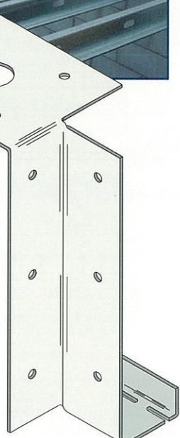
Specially designed hanger brackets allow for fast on-site fixing to either traditional brick, block or timber walls. The brackets are normally screw fixed to our joists on site. AyrJoists can support any of the flooring systems currently available. Accessories such as service hole grommets and fixing screws are available on request.
