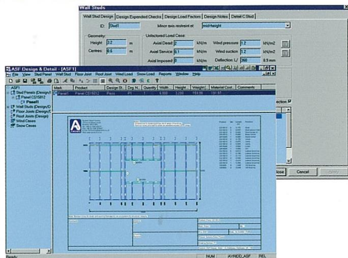
**ASF Design and Detail** is the program to be used in conjunction with this manual, and Ayrshire Steel Framing in general. The program can be used to generate hard copies, and electronic records of specific design projects, panel detail drawings including openings and priced bills of materials. The program includes access to our unique wind and snow analysis software, based on BS6399:Part 2:1997 - including latest amendments: March 2002.
