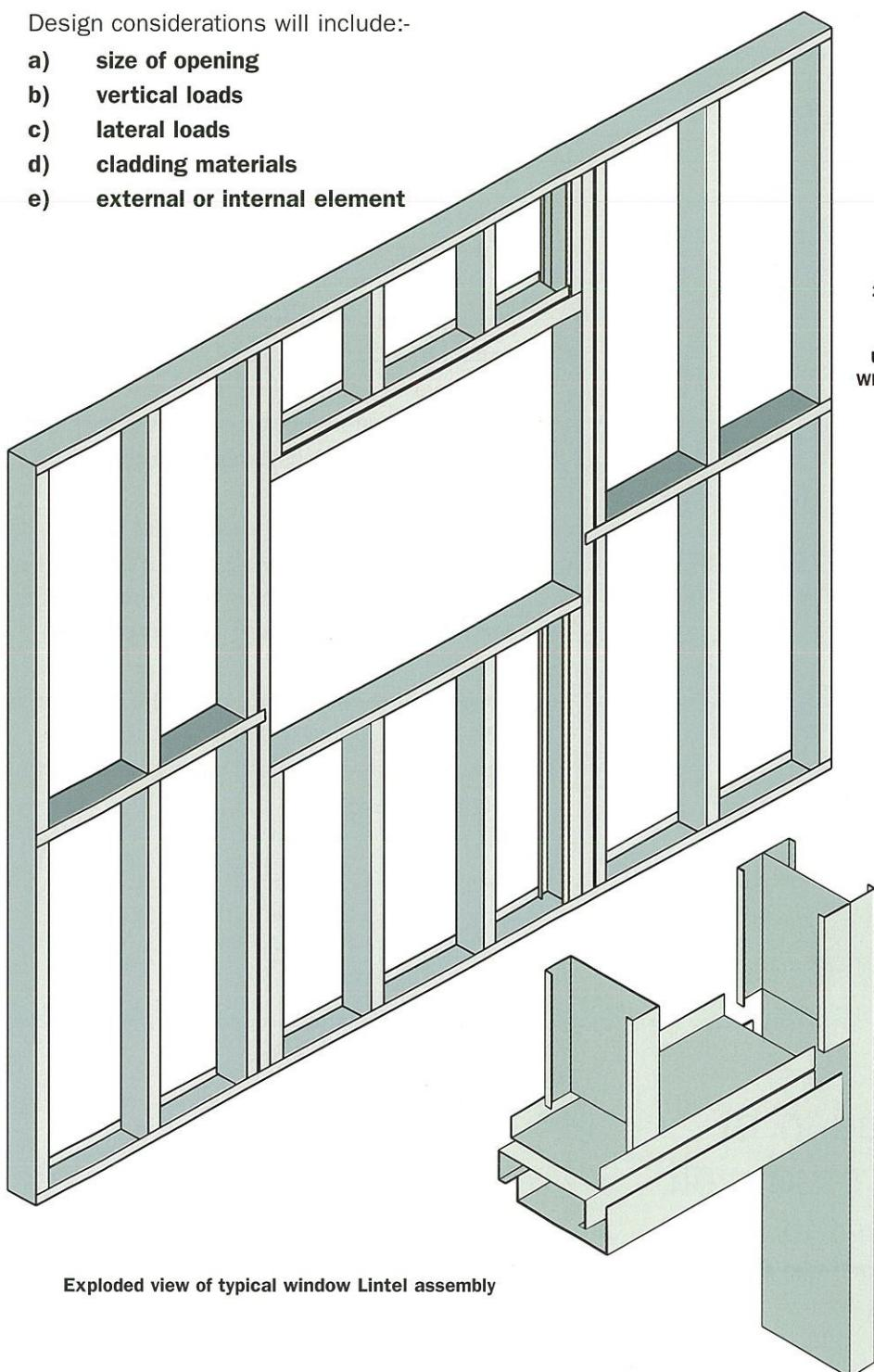
Exploded view of typical window Lintel assembly
