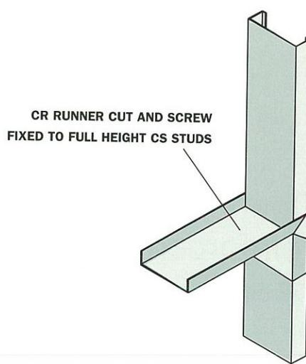
Larger openings may also require CS studs to be fitted back to back as shown here.
