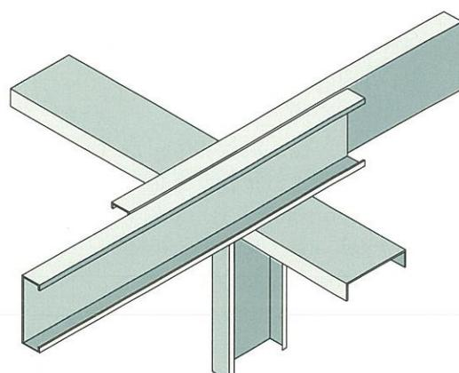
**Continuous span - joist reinforcement over load bearing stud wall or beam**
